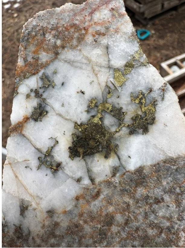
Figure 2 – Nonmagnetic sulfide (I) vein mineralization. 17.60 g/t Au and 0.09 \times 10^{-3} K SI
