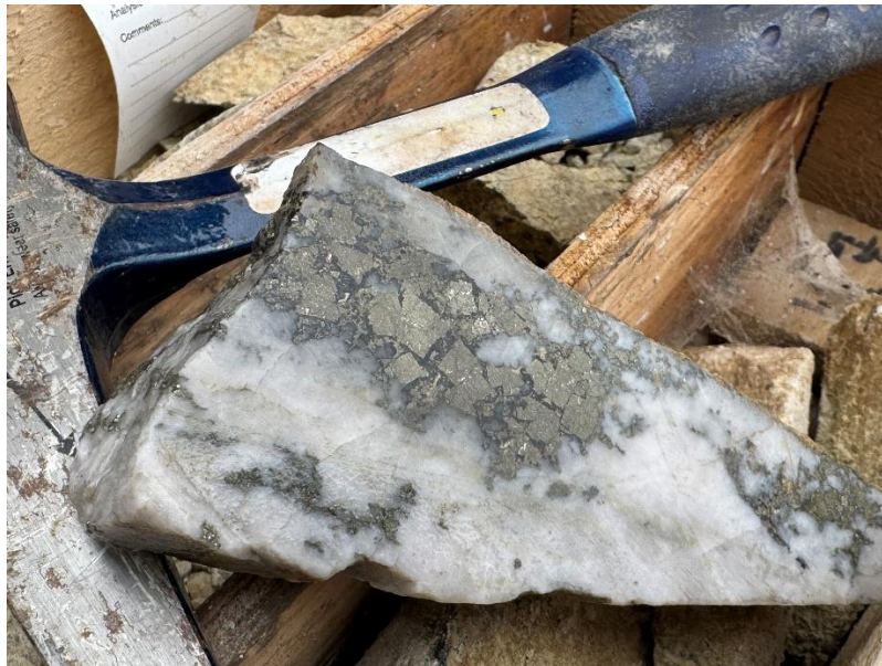
Figure 3 – Magnetic sulfide (II) vein mineralization. 9.11 g/t Au and 143 \times 10^{-3} K SI
